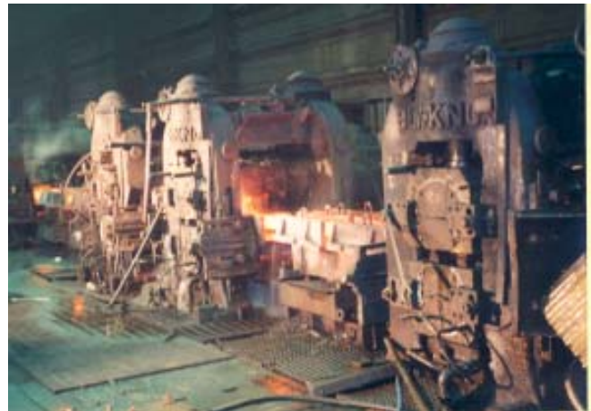
Descaled billets move through forming dies.
