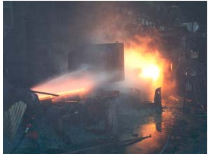
High-pressure water quickly and efficiently removes scale from steel billets.
