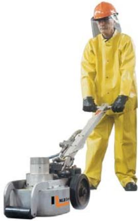
**Semi-automated** equipment often features rotating water jet nozzles (e.g., NLB's patented SPIN JET®) to maximize cleaning power. These are commonly mounted in a lawnmower-style unit that an operator can easily maneuver over a floor or grate. They are not pushed, but guided... a task that is even easier with NLB's lightweight aluminum models. Adjustable spray patterns (two or four nozzles, variable angles) allow users to use a single unit for different applications.
